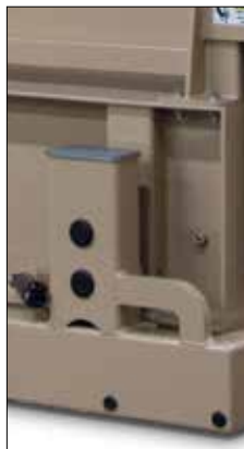
Load cell enclosure
