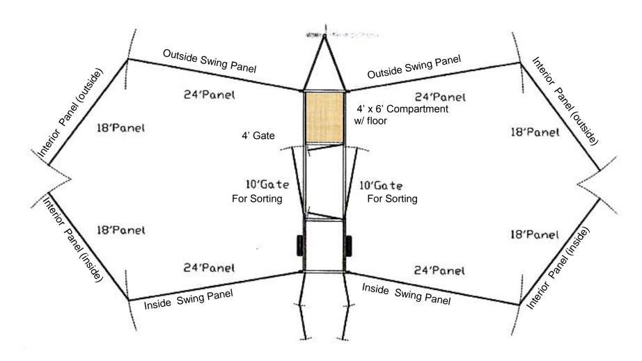
80 to 100 Cow Capacity. Sort with ease between a single pen on either side of the loadout alley! Unique front compartment hauls an atv, livestock, or supplies. Features a 7-bar panels and gates (1-1/2" square tubing, 14 gauge steel).
