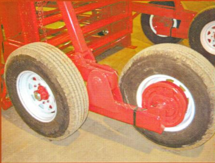
Walking I-beam carries the weight of the unit on rough ground. Electric brakes are on all four wheels.
