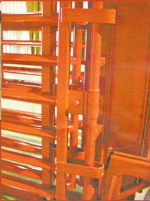
Splitting goose-neck hitch gives you the ability to load cattle out the front of the unit.
