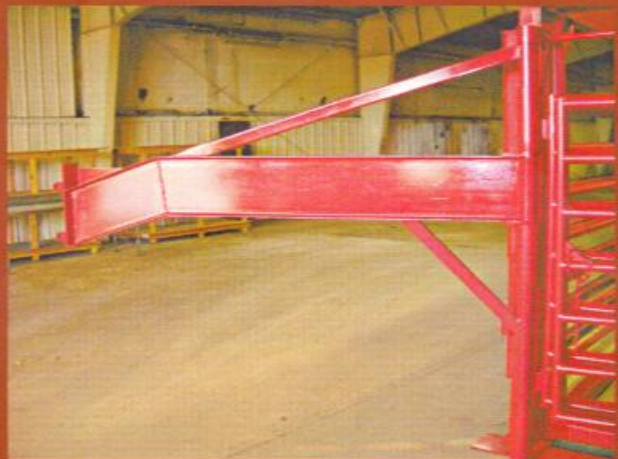
Splitting goose-neck hitch gives you the ability to load cattle out the front of the unit.
