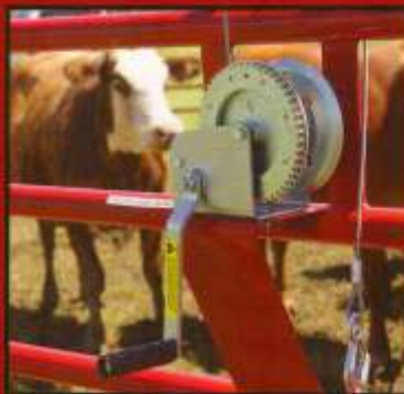
Panels lifted with winches.
